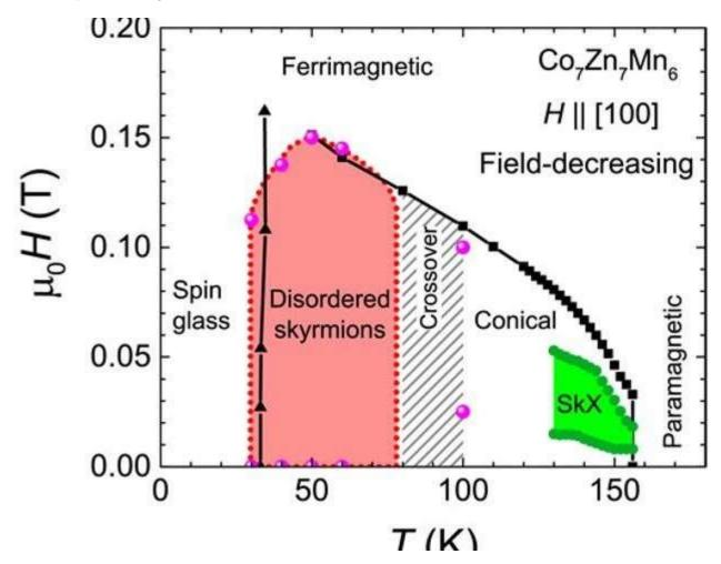
Temperature-field phase diagrams in Co7Zn7Mn6. The field-decreasing runs from the induced ferromagnetic region down to the zero-field cooling (ZFC) depicted. The phase boundaries of conventional SkX phases are seen in green circles. The ...more
