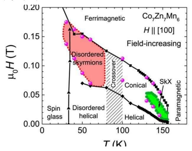
Temperature-field phase diagrams in Co7Zn7Mn6. Magnetic-field (T-H) phase diagrams in Co7Zn7Mn6 determined by ac susceptibility and SANS measurements. Field-increasing runs after zero-field cooling (ZFC) depicted. The conventional SkX field ...more
