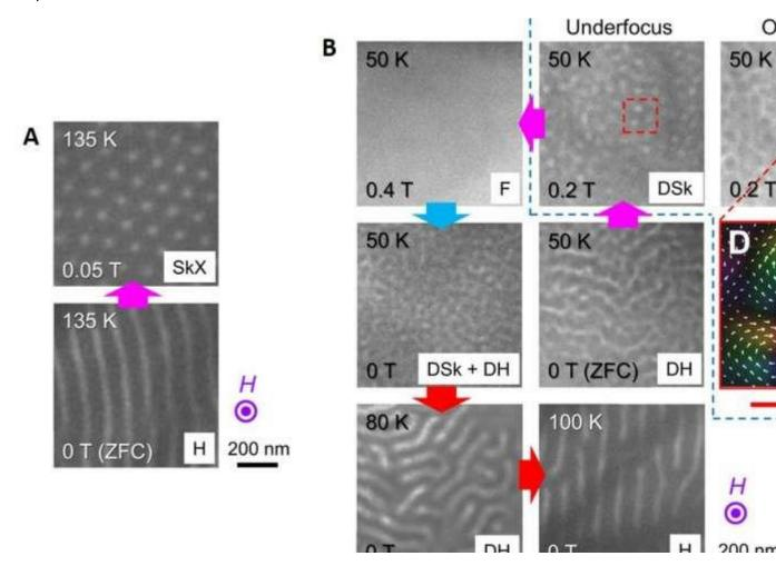
LTEM measurement on a thin-plate sample of Co7Zn7Mn6. A) underfocused LTEM images at 135 K and at 0 T and 0.05 T. B) Underfocused LTEM images at selected fields at 50 K and at selected temperatures in the subsequent zero-field warming (ZFW) ...more
