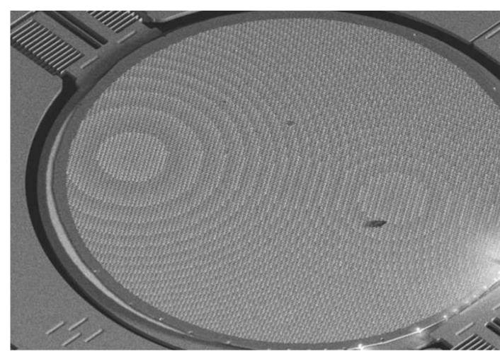
In this image, a circular metasurface-based flat lens has been integrated onto a MEMS scanner. Integration of MEMS devices with metalenses combine the strength of high-speed dynamic control with precise spatial manipulation of wave-fronts. ...more
