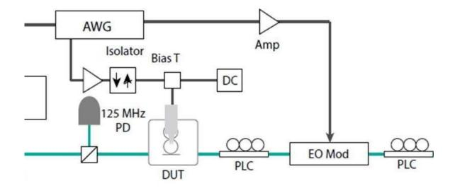
Extended experimental setup. The device is optically pumped by a tunable telecom laser centered around 1630 nm. The light is sent through an external electro-optic modulator and polarization controllers (PLC) before coupling into the chip ...more
