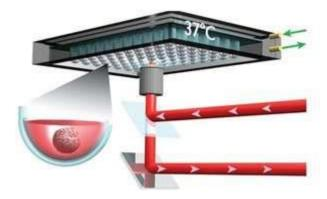
A multiwell plate where each well contains tumor tissue is placed on an inverted microscope held at 37°C. A laser beam is focused on one area of the tumor, then moved to achieve a mapping. The diffused light is collected by the microscope ...more
