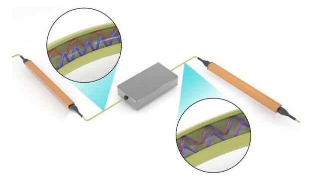
The researchers' innovative experimental setup involved operating on photons contained within a single fiber-optic cable. This provided stability and control for operations producing entangled photons, shown separated at top and intertwined ...<u>more</u>"We were able to extract more information about the quantum state of our experimental system using Bayesian inference than if we had used more common statistical methods," Williams said.
