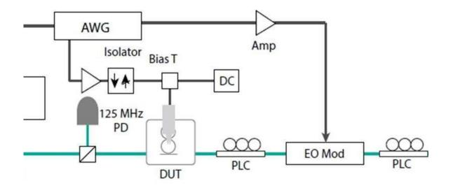
Extended experimental setup. The device is optically pumped by a tunable telecom laser centered around 1630 nm. The light is sent through an external electro-optic modulator and polarization controllers (PLC) before coupling into the chip ...<u>more</u>
