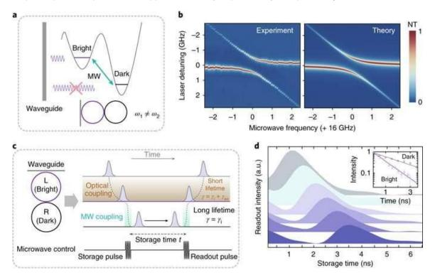
On-demand storage and retrieval of light using a photonic dark mode. a) The photonic molecule is programmed to result in localized bright and dark modes. As a result, the bright mode can be accessed from the optical waveguide, while the ...<u>more</u>
