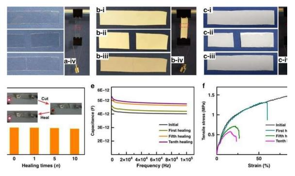
Characterizing the EL device. a–c) Images of the self-healing processes of the EL component layers and the device (PAA layer—a, PU composite layer—b, and EL device—c). In these processes, i) shows the initial states, ii) shows the cut ...<u>more</u>
