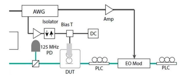
Extended experimental setup. The device is optically pumped by a tunable telecom laser centered around 1630 nm. The light is sent through an external electro-optic modulator and polarization controllers (PLC) before coupling into the chip ...<u>more</u>
