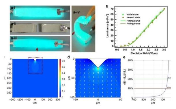
Characterizing the initial healing response: light-emitting performance of the self-healed EL device after cutting-healing process. a Demonstration of cutting-healing process of the healable EL device. a-i-a-iii exhibits the initial working ...more
