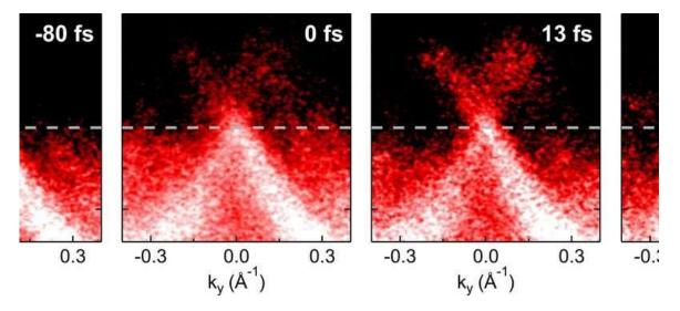
Film recordings show for the first time how the energy distribution in a graphite sample changes in the ultrashort period of 50 femtoseconds. Credit: Phys. Rev. Lett
