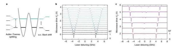
Microwave dressed photonic waveguides. a) When the applied microwave frequency is tuned to match the mode separation, dissipative coupling leads the two photonic levels to split into four levels. This effect is analogous to Autler–Townes ...more
