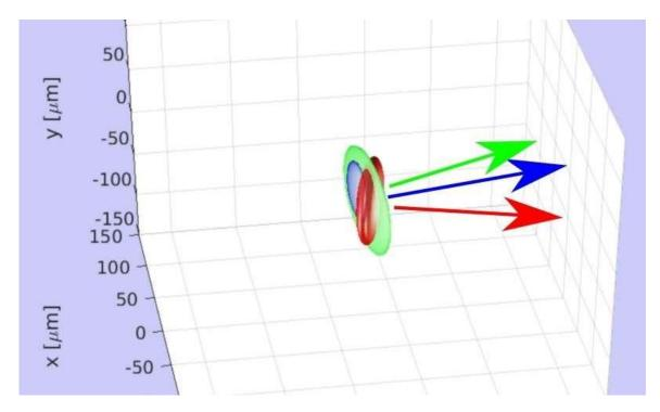
With the Hussar program, you can now efficiently model the interactions of femtosecond laser pulses travelling at a mutual angle of up to 140 degrees. Credit: IPC PAS
