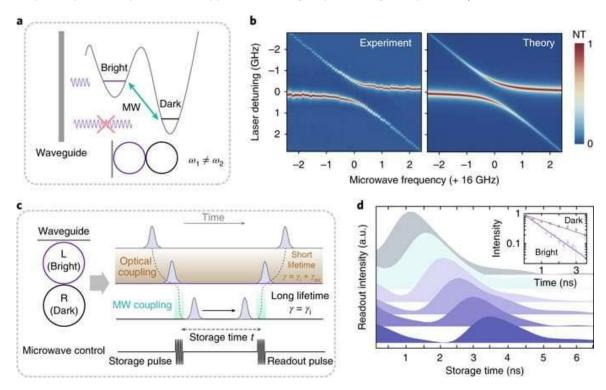
On-demand storage and retrieval of light using a photonic dark mode. a) The photonic molecule is programmed to result in localized bright and dark modes. As a result, the bright mode can be accessed from the optical waveguide, while the ...more
