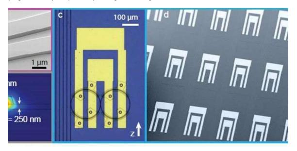
Device and experimental setup detail. a) Scanning electron microscope (SEM) image of the gap between the coupled microring resonators. b) Cross-section of the optical mode profile in the ring resonator. c) Microring image of the full device ...more
