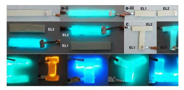
LEGO assembly process of self-healing EL devices. a) A complete EL device was cut into two individual EL units. a-i) indicates the initial resting state, a-ii) the working state, and a-iii) the cut state. b) The as-obtained two EL units in ...more
