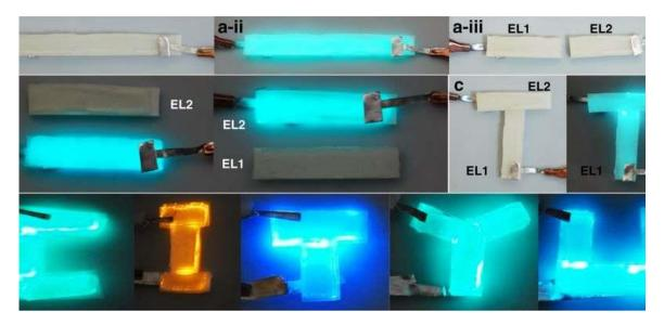
LEGO assembly process of self-healing EL devices. a) A complete EL device was cut into two individual EL units. a-i) indicates the initial resting state, a-ii) the working state, and a-iii) the cut state. b) The as-obtained two EL units in ...<u>more</u>
