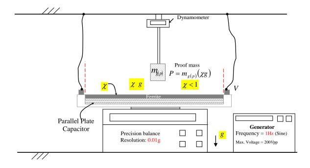
Fig. 1 – Experimental set up for controlling the *Gravitational Mass* of the Ferrite Lamina, and the *Gravity* acceleration above it. Note that the Ferrite Lamina has inertial mass  $m_{i(ferrite)} = 0.20 \times 0.20 \times 2 \times 10^{-3} \times 5000 = 0.4 kg$ . Thus, the precision balance must have resolution of 0.01g or less.
