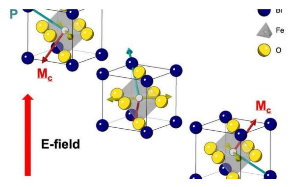
Single crystals of the multiferroic material bismuth-iron-oxide. The bismuth atoms (blue) form a cubic lattice with oxygen atoms (yellow) at each face of the cube and an iron atom (gray) near the center. The somewhat off-center iron ...moreInternet of things and AI
