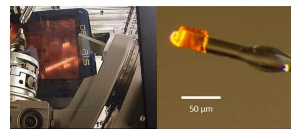
On the left is the gyroscope, designed to rotate the crystal through a series of different angles as the X-ray beam hits it. Behind it is the detector panel which records the diffraction spots. On the right is a zoomed in picture of a ...more
