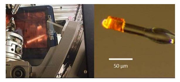
On the left is the gyroscope, designed to rotate the crystal through a series of different angles as the X-ray beam hits it. Behind it is the detector panel which records the diffraction spots. On the right is a zoomed in picture of a ...<u>more</u>
