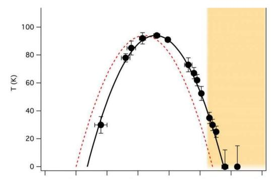
This phase diagram for BSCCO plots the temperature (T, in degrees Kelvin, on the y axis) at which superconductivity sets in as more and more charge vacancies, or "holes," are doped into the material (horizontal, x axis). On the underdoped ...<u>more</u>"Until this study, nothing past that point was known because we couldn't get crystals doped above that level. But our new data takes us to a point of doping way beyond the previous limit, to a point where Tc is not measurable."
