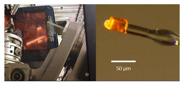
On the left is the gyroscope, designed to rotate the crystal through a series of different angles as the X-ray beam hits it. Behind it is the detector panel which records the diffraction spots. On the right is a zoomed in picture of a ...more
