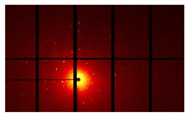
This is a diffraction pattern that results when you shoot an X-ray beam at a single crystal. Credit: Kerry Rippy, <u>CC BY-ND</u>
