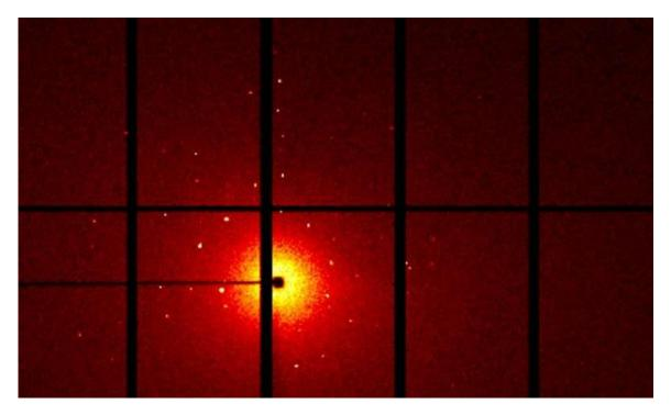
This is a diffraction pattern that results when you shoot an X-ray beam at a single crystal. Credit: Kerry Rippy, <u>CC BY-ND</u>
