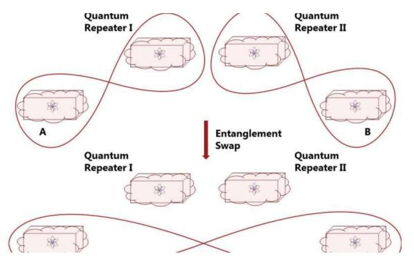
Illustration: When distributing entanglement between sender A and receiver B, the communication line is segmented by inserting quantum repeaters. In this illustration A is entangled with Quantum Repeater I while B is entangled with Quantum ...more
