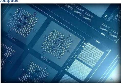
Layout of IBM's four superconducting quantum bit device. Using a square lattice, IBM is able to detect both types of quantum errors for the first time. This is the best configuration to add more qubits to scale to larger systems.
