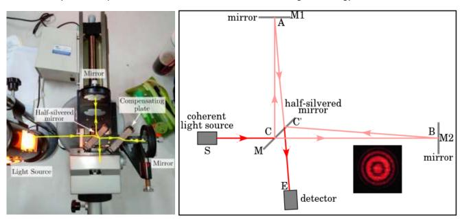
Figure 45: Michelson Interferometer setup: parallel merged beams
