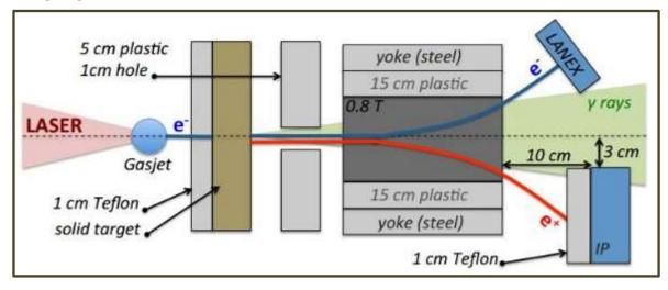
Figure 9: Laser Generated Electron and Positron Generation Setup
