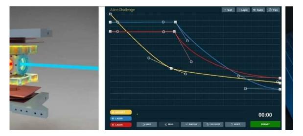
Game interface of the Alice Challenge. Players could manipulate three curves representing two laser beam intensities and the strength of a magnetic field gradient, respectively. The chosen curves were then realized in the laboratory in real-time. Credit: Robert Heck, AU**The RedCRAB package**
