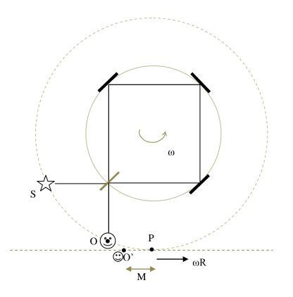
First we get the expression of the time *t* required for the observer O to move from its current position, point O,( position at instant of light emission, t = 0) to point P. This will be the length of arc OP divided by the tangential velocity of the observer.
