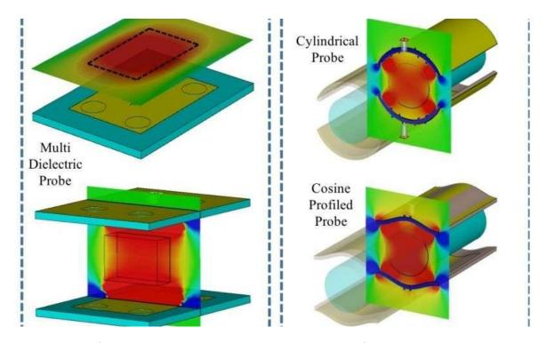
Proposed radio frequency probes to create homogeneous magnetic field within a phantom under study: single multi dielectric patch surface probe (upper left), volume probe composed of two vis-à-vis placed dielectric patch probes (lower left), ...more
