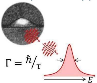
A single-photon source never emits two or more photons at the same time. Single photons are important in the field of quantum information technology where, for example, they are used in quantum computers. Alongside the brightness and robustness of the light source, the indistinguishability of the photons is especially crucial. In particular, this means that all photons
