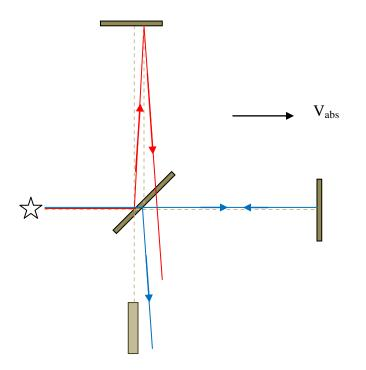
We can see from the above diagram that, even in the reference frame of the MMX apparatus, the transverse light beam (red line) will be bent forward on reflection from the beam splitter due to motion of the apparatus relative to the ether and there would be no interference pattern because the two light beams will not meet at the point of detection. The transverse light beam will miss the detector.
