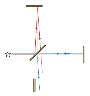
We can see from the above diagram that, even in the reference frame of the MMX apparatus, the transverse light beam (red line) will be bent forward on reflection from the beam splitter due to
