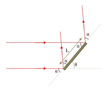
Next consider light reflection from a mirror that is moving to the right with velocity  $V_{abs}$  in the ether.
