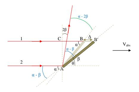
Therefore, the effective angle of incidence is  $\alpha$ - $\beta$ . The angle of reflection should also be  $\alpha$ - $\beta$ . Relative to the actual mirror ( in the reference frame of the mirror ), the angle of incidence is  $\alpha$  and the angle of reflection is  $\alpha$  -  $2\beta$ !
