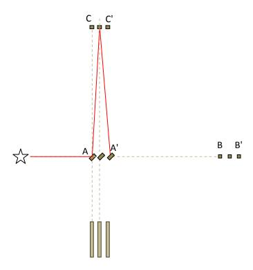
Light from the source hits the beam splitter at point A. The standard analysis starts from the assumption that the transverse light beam will not miss the detector. With this assumption, in the time interval that the beam splitter moves from A to A', the transverse light beam will make round trip time, to meet the beam splitter at point A'.
