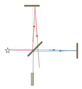
We can see from the above diagram that, even in the reference frame of the MMX apparatus, the transverse light beam ( red line ) will be bent forward on reflection from the beam splitter due to
