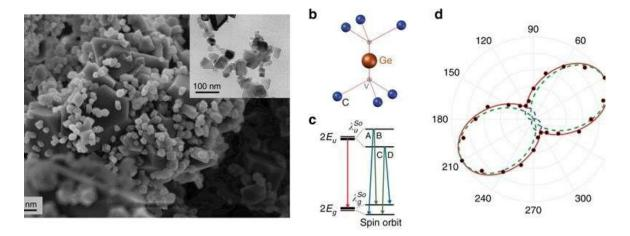
Characterization of the nanodiamonds: a) SEM images of the GeV nano and microdiamonds of the raw sample after HPHT synthesis, the TEM image is seen inset. b) the Ge atom is located in the middle of two empty lattice sites, which includes ...more
