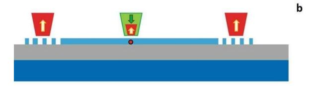
On-chip excitation of a single GeV nanodiamond (ND) assigned via controlled placement in a device fabricated with hydrogen silsesquioxane (HSQ) atop Ag film a) the sample layout and working principle of direct excitation of a GeV ...more
