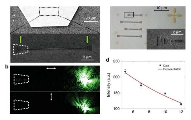
Transmission of green laser light (532 nm) along the low-loss plasmonic waveguide, a) SEM image of a single crystalline flake (top) and fabricated DLSPP waveguide atop of the Ag plate (bottom), b) optical characterization of the waveguide ...more
