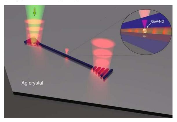
Schematic illustration of the device layout and working principle for on-chip excitation of a nanodiamond. The nanodiamond carries spectrally narrow single GeV quantum emitters embedded in a DLSPP waveguide. Credit: Light Science & Applications, doi: 10.1038/s41377-018-0062-5.
