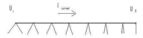
Figure 1.) Aluminium folios shows the charge distribution on the electric wire
