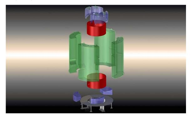
A diagram showing the components of the acrylic tanks veto system for the LUX-ZEPLIN experiment. The green and blue objects represent the clear acrylic tanks. They will be fitted snugly together and held by a metal base. Credit: LZ Collaboration
