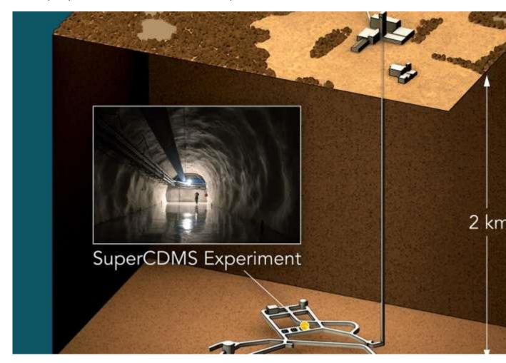
The SuperCDMS dark matter experiment will be located at the Canadian laboratory SNOLAB, 2 kilometers (6,800 feet) underground inside a nickel mine near the city of Sudbury. It's the deepest underground laboratory in North America. There it ...<u>more</u>
