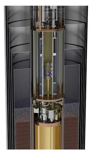
A cutaway rendering of the ADMX detector, which can detect axions producing photons within its cold, dark interior. Credit: ADMX collaboration
