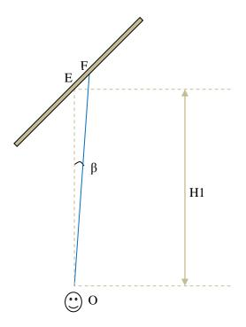
We can easily see that angle E is equal to  $135^{\circ}$  (because the beam splitter has  $45^{\circ}$  inclination). Therefore, angle F will be equal to  $180^{\circ} - 135^{\circ} - \beta = 45^{\circ} - \beta$ .
