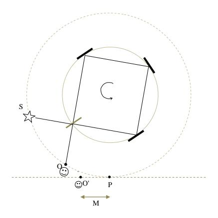
The second expression for t is obtained from the requirement that imaginary inertial observer O' will also move from point O' to point P during this time interval, t.
