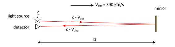
According to Apparent Source Theory, since the source and the detector are located almost at the same point in space, absolute motion of the system will not have any effect[1], and we simply apply emission theory regarding the group velocity, which is relevant in this experiment, because this is a time of flight experiment.
