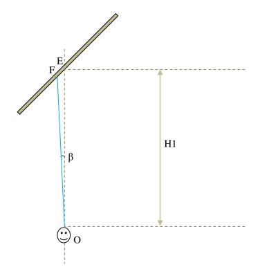
Angle E is equal to  $45^{\circ}$  (because the beam splitter has  $45^{\circ}$  inclination).
