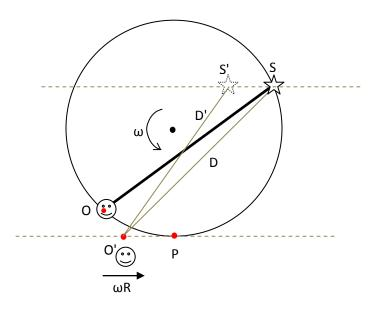
The above setup is more general in which the source and observer are rotating about a center that is not on the line connecting them and requires more involved analysis. A simpler case in which the center of rotation is on the middle point of line OS, as shown below.
