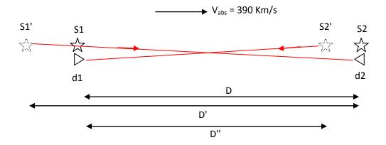
According to Apparent Source Theory, D' is the distance of apparent source S1' relative to detector d2 and D" is the distance of apparent source S2' relative to detector d1, and
