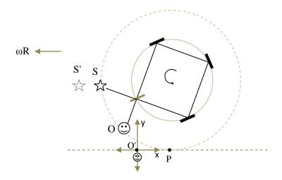
The problem is therefore solved in the reference frame of imaginary inertial observer O'. For this, as already mentioned, the positions and motions of the beam splitter and the mirrors should be described in the reference frame of observer O'. Note that, the motion of the beam splitter and the mirrors in the reference frame of O' is a combination of translational and rotational motions.
