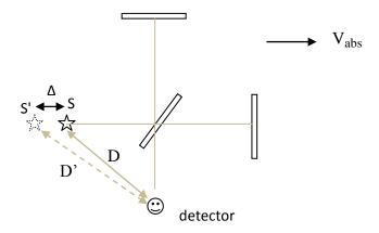
According to Apparent Source Theory, there will be an apparent change in position of the light source as seen by the detector. The apparent change in source position is determined by the source-detector  $\underline{\text{direct}}$  distance D, the magnitude and direction of the absolute velocity  $V_{abs}$ .
