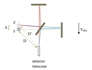
We can see from the diagram above that, according to AST, the effect of absolute motion is not only to create a change in path difference but also misalignment of the two light beams.
