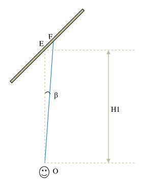
We can easily see that angle E is equal to  $135^0$  (because the beam splitter has  $45^0$  inclination). Therefore, angle F will be equal to  $180^0$  -  $135^0$  -  $\beta = 45^0$  -  $\beta$ .
