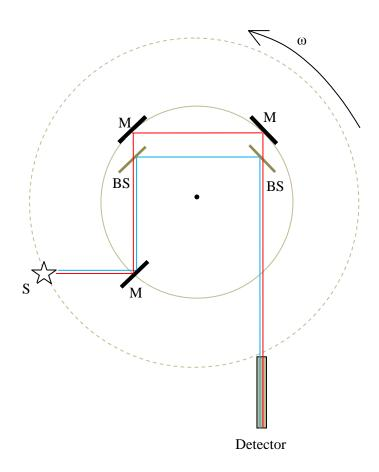
Here we propose a modified Sagnac experiment in which two light beams propagate in the same direction ( CW or CCW ) , instead of in opposite directions, as shown above. M represents mirror and BS represents beam splitter.
