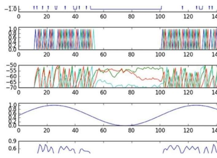
Results of the experiment controlling oscillation in the phase space defined by a single principal component. The first plot from the top is a plot of the input into the actuated cell over time; the second plot from the top is a plot of ...**more**
