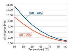
Fig. 1: Wind speed over a warm water surface to blow away the generated steam (30 kg/h).
