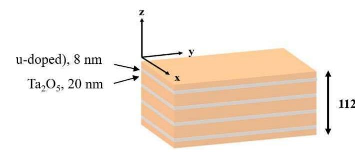
Cross-sectional view of the hyperbolic metamaterial examined in the new study shows layers of copper-doped silver and tantalum pentoxide. Credit: NIST
