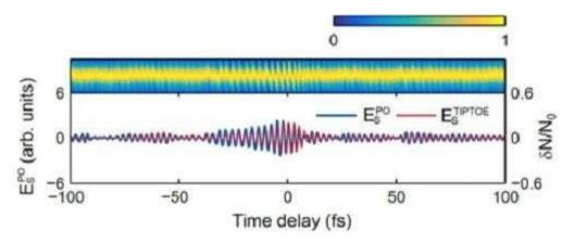
Comparison between attosecond X-ray pulse method X-ray (blue) and TIPTOE (red) to validate the new technique developed by IBS scientists. The waveforms measured with TIPTOE match the ones obtained with the conventional method. Credit: Institute for Basic Science
