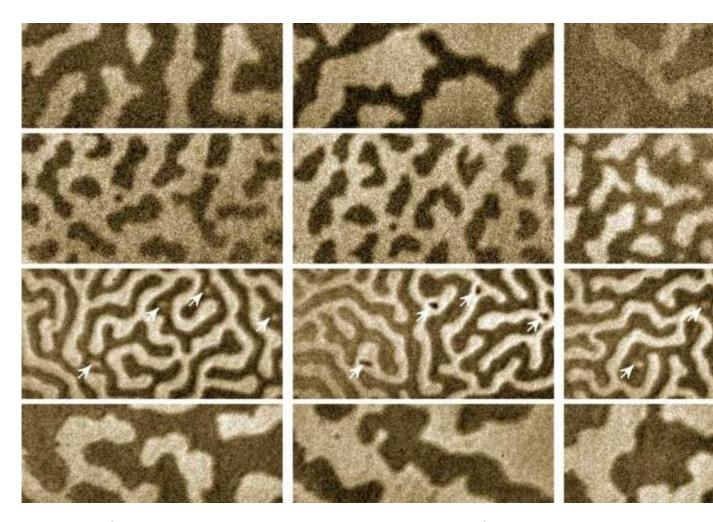
In these rows of sequenced images, produced using X-ray-based techniques, the first column shows the demagnetized state of a multilayer material containing gadolinium and cobalt; the second column shows the residual magnetism in the same ...more
