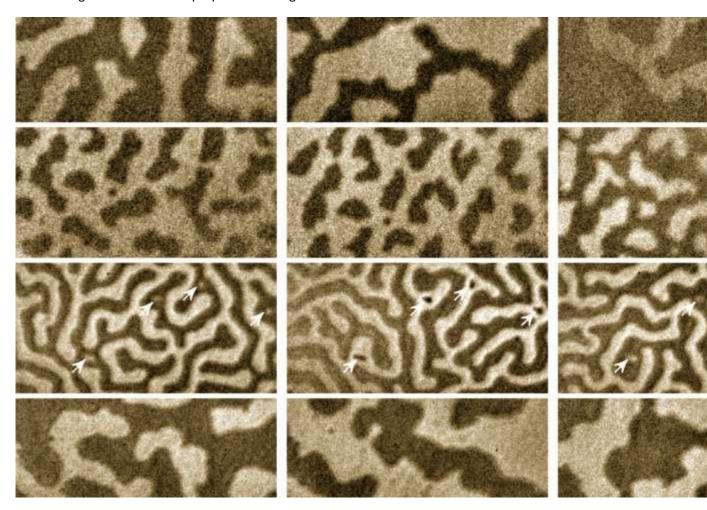
In these rows of sequenced images, produced using X-ray-based techniques, the first column shows the demagnetized state of a multilayer material containing gadolinium and cobalt; the second column shows the residual magnetism in the same ...more
