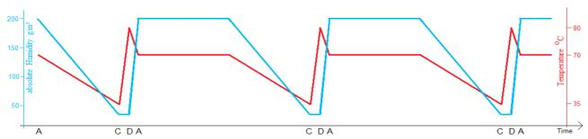
Fig. 5: Changes in the temperature and water content of a small air volume  $(10^{-3} \text{ m}^3)$  during the circulation in the improved concentric condenser. The letters on the horizontal axis refer to Fig. 2
