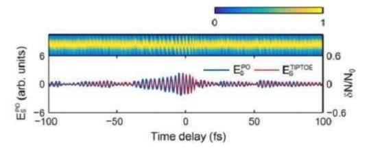
Comparison between attosecond X-ray pulse method X-ray (blue) and TIPTOE (red) to validate the new technique developed by IBS scientists. The waveforms measured with TIPTOE match the ones obtained with the conventional method. Credit: Institute for Basic Science
