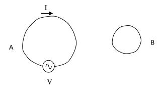
We know that a DC current in the first coil (A) will have no effect on the second coil(B). However, if the current in the first coil is varying with time, a time varying magnetic field will be created, which will produce voltage and current in the second coil. The current in the second coil will, in turn, create back EMF on the first coil, thereby *reacting to (opposing ) the change in current in the first coil*.
