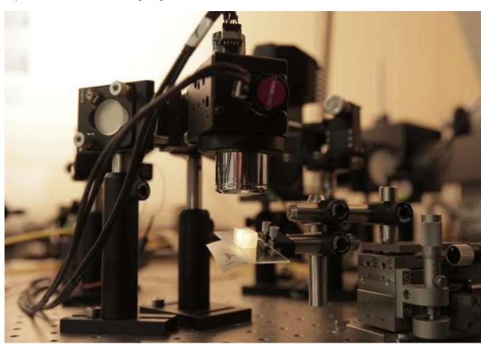
This custom-built optical coherence tomography instrument uses visible light to view tissue. Credit: Renee Meiller
