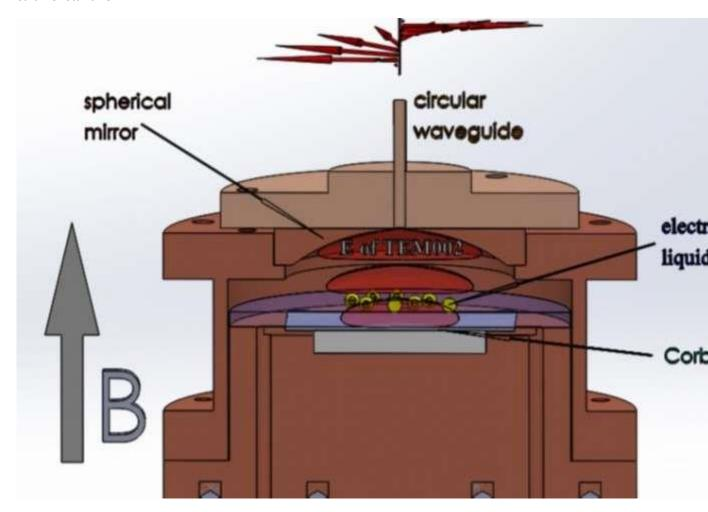
Custom-designed vacuum chamber that contains electrons above the condensed helium. The microwaves are introduced into the chamber through a waveguide and focused onto the electrons by a spherical mirror. Credit: OIST
