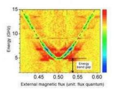
An energy band gap is obtained using energy spectroscopy. Existence of band gap establishes that coherent tunneling has occurred. Credit: RIKEN
