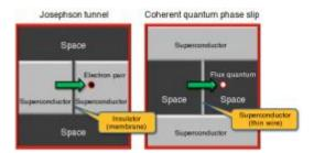
This figure shows the Josephson tunnel (left) and coherent quantum phase slip (right). At left, two superconductors are separated by thin insulator (in this case space). A current is produced by superconducting electron pairs tunneling ...more
