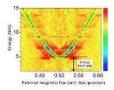
An energy band gap is obtained using energy spectroscopy. Existence of band gap establishes that coherent tunneling has occurred. Credit: RIKEN
