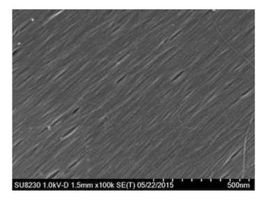
A scanning electron microscope image shows highly aligned and closely packed carbon nanotubes gathered into a film by researchers at Rice. Credit: Kono Laboratory
