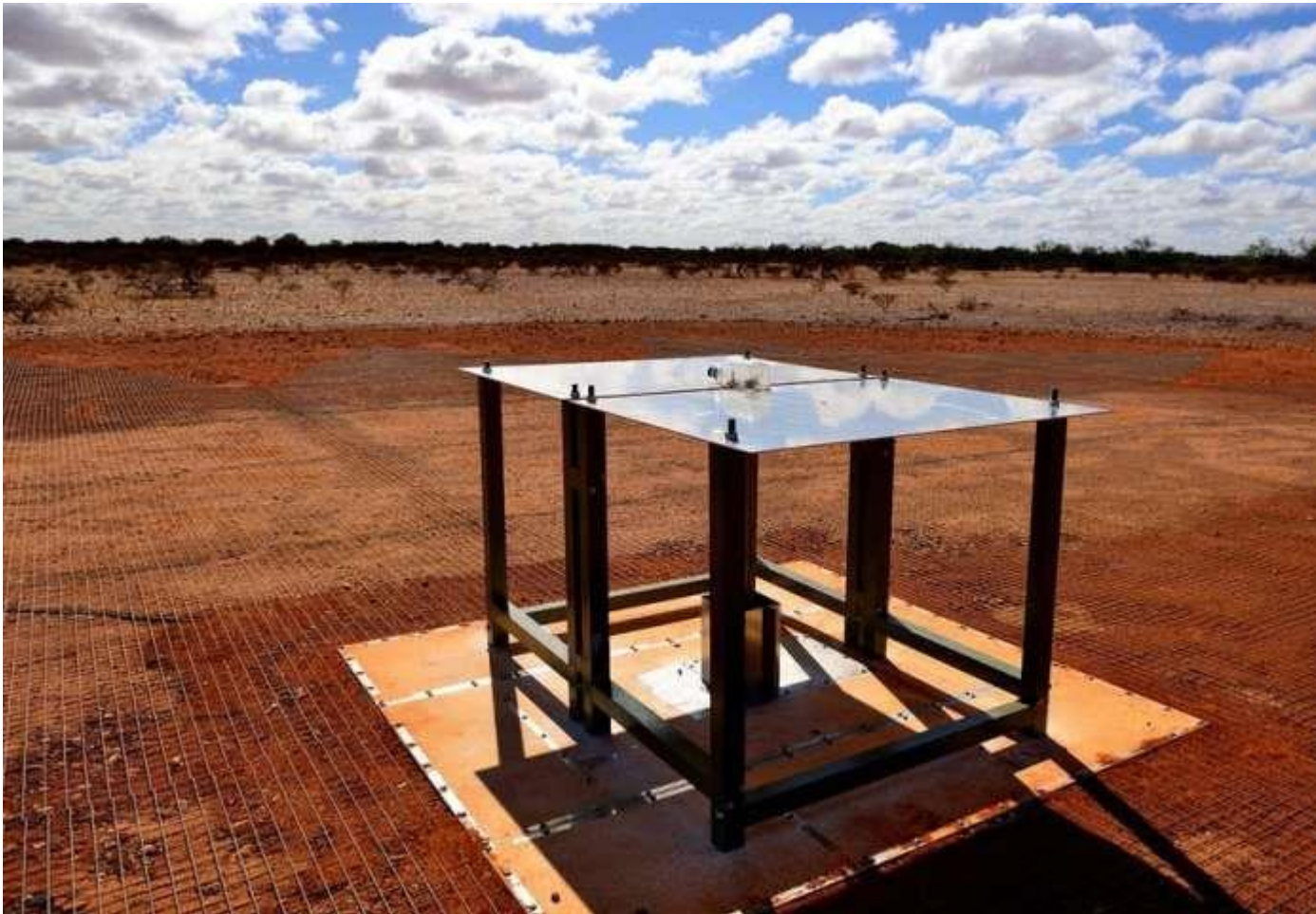
The EDGES ground-based radio spectrometer, CSIRO's Murchison Radio-astronomy Observatory in Western Australia. Credit: CSIRO
